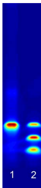
Figure S4. Lane 2 is the mixture of the HPLC purified Cy3-labelled poly-dT 10-mer, 15-mer and 20-mer (all ordered from IDT). Lane 1 is the 5'-Cy3-labeled poly-dT 20-mer sample we synthesized from the PFPE microfluidic chip, without purification.
