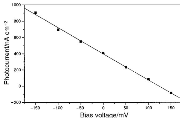
**Fig. 7** Photocurrent versus bias voltage for a Crown D-ITO electrode in 0.1 M NaCl aqueous solution under ambient conditions, upon irradiation with 137 mW cm<sup>-2</sup> white light.
