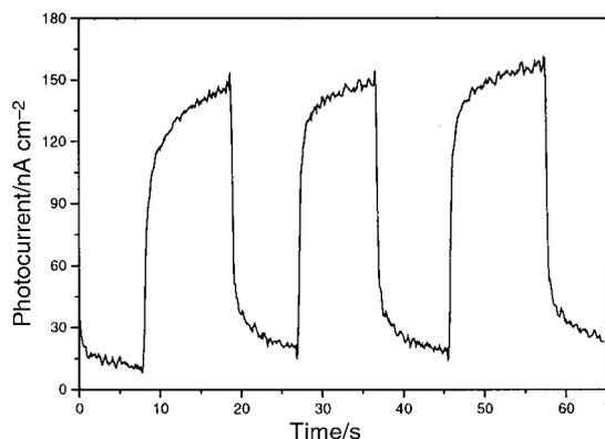
**Fig. 6** Photocurrent generation of Crown D-ITO electrode deposited from pure water subphase in 0.1 M Bu<sub>4</sub>NBr electrolyte solution under ambient conditions, upon irradiation with 137 mW cm<sup>-2</sup> white light.
