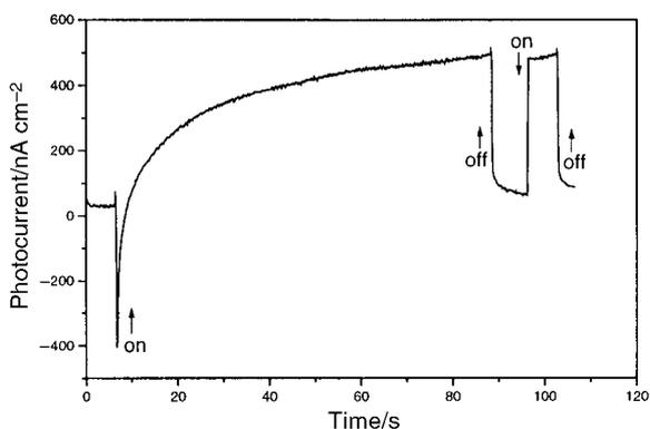
**Fig. 4** The photoelectric response of a Crown D-ITO film deposited from pure water subphase in 0.1 M NaCl electrolyte solution under ambient conditions, upon irradiation with  $137 \text{ mW cm}^{-2}$  white light.
