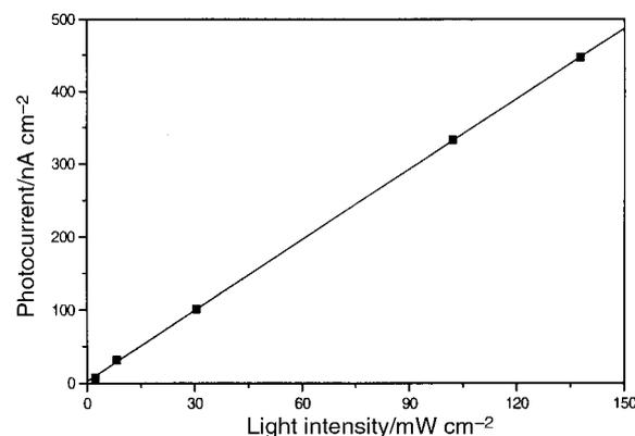
**Fig. 8** Dependence of the photocurrent on light intensity for a Crown D-ITO electrode in 0.1 M NaCl electrolyte solution under ambient condition without bias voltage.
