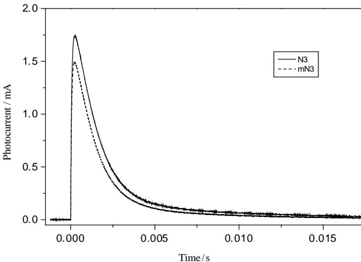
Fig. 7. Time-dependent photocurrent decay curves for solar cells sensitized by N3 and mN3, respectively. Illuminated from the substrate side with 532 nm laser ( $23 \mu\text{J pulse}^{-1}$ ).
