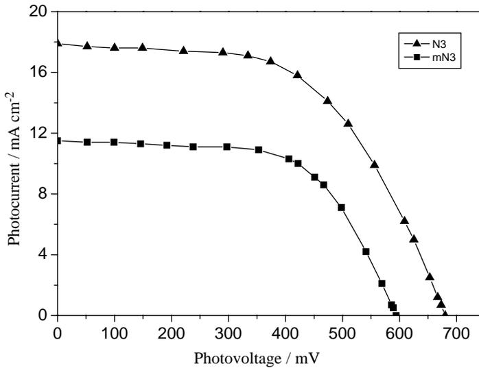
Fig. 5. The  $I-V$  curves for N3 and mN3. Solar cells were illuminated under white light of  $89.5 \text{ mW cm}^{-2}$  from a xenon lamp.
