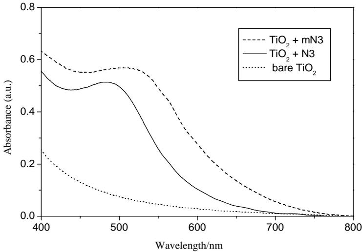
Fig. 3. UV-vis spectra for N3 and mN3 on TiO<sub>2</sub> films, and for bare TiO<sub>2</sub> films, respectively. TiO<sub>2</sub> films used here were about 4 μm thick. Absorption of CTO glass was deducted.
