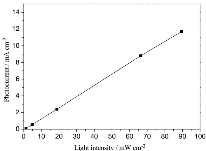
Fig. 6. Relationship between light intensity and the short-circuit photocurrent generated by mN3-sensitized solar cells.
