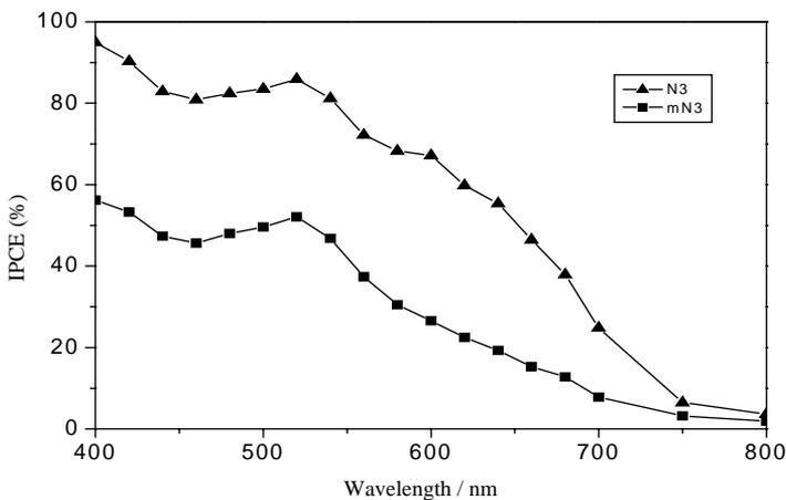
Fig. 4. Photocurrent action spectra for N3 and mN3. IPCE was corrected for the absorption and reflection by CTO glass.
