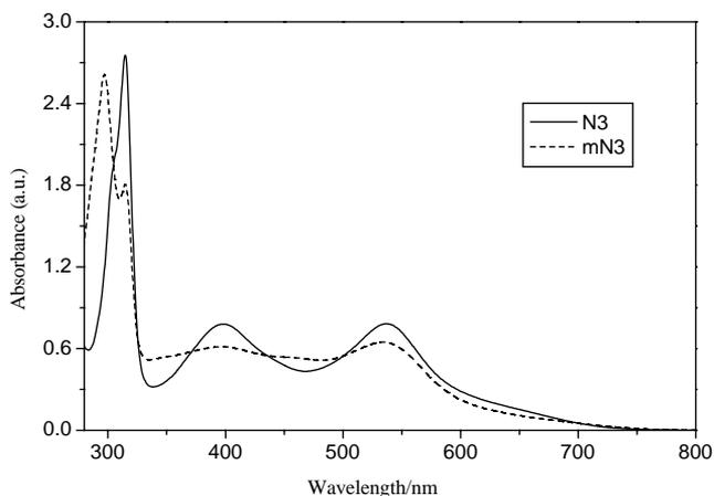
Fig. 2. UV-vis spectra for N3 and mN3 in ethanol solutions.
