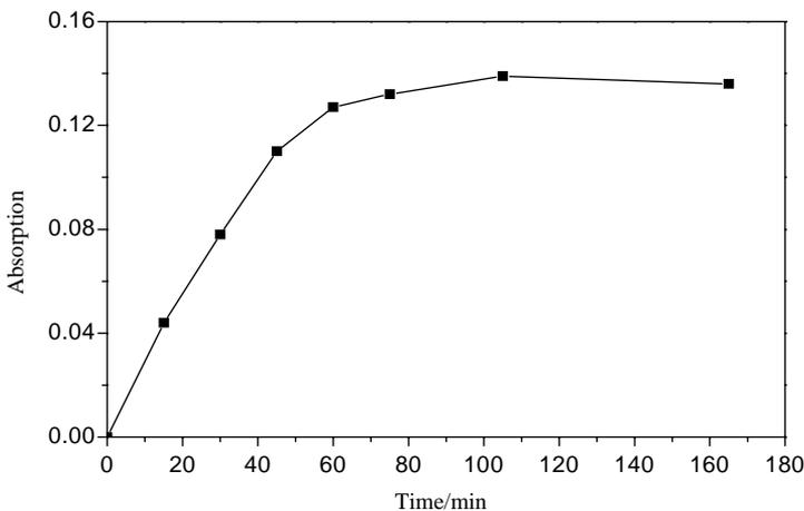
Fig. 1. Relationship of maximum absorption of mN3 and sensitization duration. TiO<sub>2</sub> films used here was about 4 μm thick. Absorption of TiO<sub>2</sub> film and glass support was deducted.
