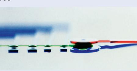
Actuation of the valves was used to determine the volume of liquid present in the chambers and thus to tune the focal length of the microlens. The researchers say that the refractive index of the microlens can be adjusted by filling the chambers with different liquids.
